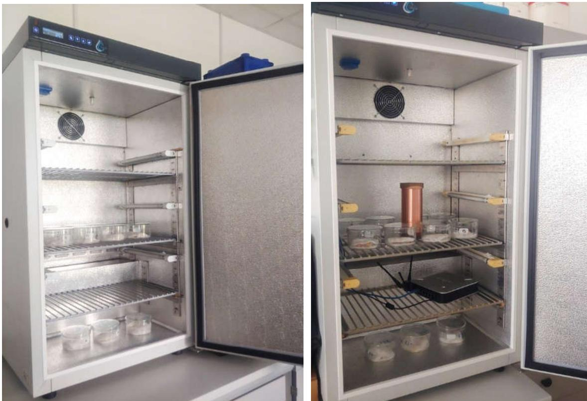
**Figure 1:** Growth chambers and arrangement of glass containers with beans. Left: control experiment, right: experiment where beans were exposed to Wi-Fi and Qi-Shield.
